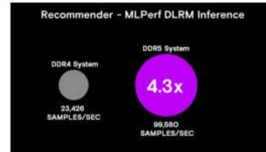
Figure 7: DLRM inferencing throughput comparison – DDR5 SYSTEM versus DDR4 SYSTEM delivers 4.3 times gain in throughput for recommendation
