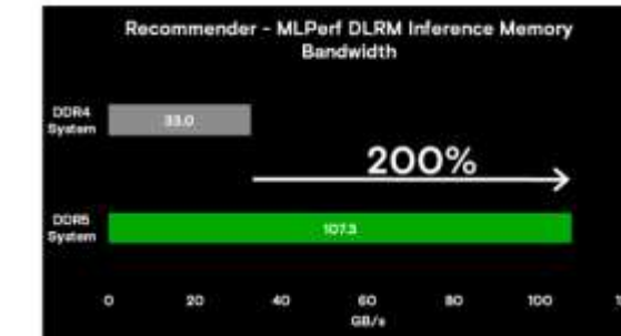
Figure 8: DLRM inferencing bandwidth comparison -DDR5 SYSTEM versus DDR4 SYSTEM provides 200% gain in memory bandwidth for recommendation
