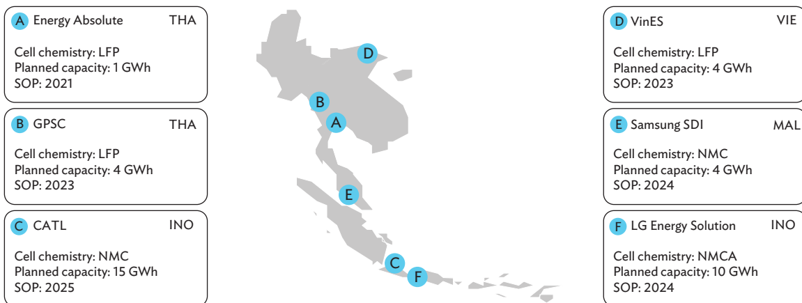
Figure 73. Announced Lithium-Ion Battery Cell Manufacturing Capacity in Southeast Asia [GWh]
