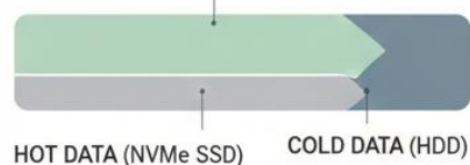
LAYERED STORAGE ARCHITECTURE
