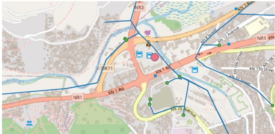
FIGURE 59. Location of the Nyabugogo Bus terminal in relation to the MV network.
